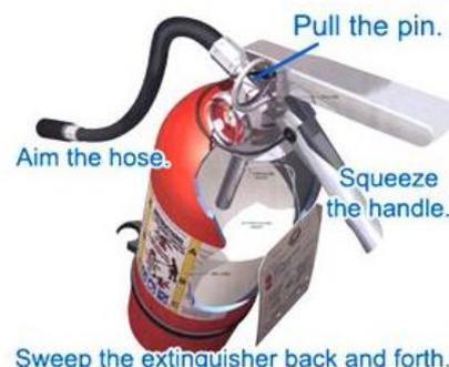
**Foam Fire Extinguishers also called AFFF FOAM** - are good for tackling fires involving flammable solids, liquids including petrol, diesel, thinners, oils, paints, wax and plastics that melt. Foam extinguishers can conduct electricity; care must be taken with regard to accidental use on exposed power cables
